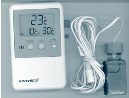
Figure 1: Min/Max Thermometer example. Note liquid filled probe.
